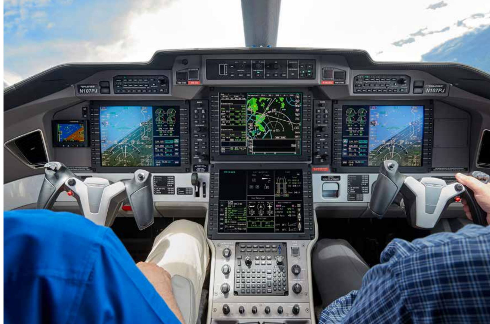
THE PC-24'S ACE (Advanced Cockpit Environment) avionics (above) is based on Version 2 of Honeywell's Epic platform. The control yoke design borrows heavily from video gaming controls. The airplane's short takeoff and landing distances make it a real performer at small, rural airports (left).
